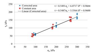
Fig. 10. Comparison of peak shearing strength parameters.
