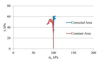
Fig. 8. Comparison of stress paths (test made according to corrected area *A*)
