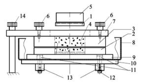
Fig. 1. Direct shear device principal constructional scheme.
