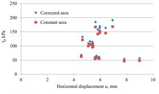
Fig. 11. Comparison of peak shearing strength versus horizontal displacement
