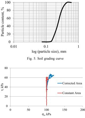
Fig. 7. Comparison of stress paths (test made according to constant area  $A_{\alpha}$ )
