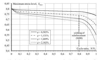
Fig. 9. Evolution of maximum stress level with number of cycles regarding to reinforcement ratio
