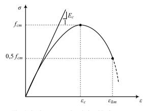
Fig. 1. Static stress-strain relationship for concrete in compression
