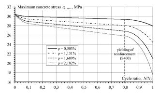
Fig. 8. Evolution of maximum stress with number of cycles regarding to reinforcement ratio
