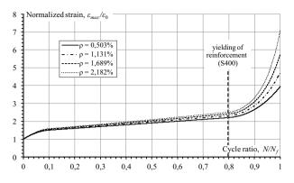
Fig. 7. Evolution of longitudinal strain with number of cycles regarding to reinforcement ratio
