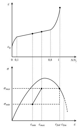
Fig. 2. Theoretical model (according to Zanuy et al. 2009)
