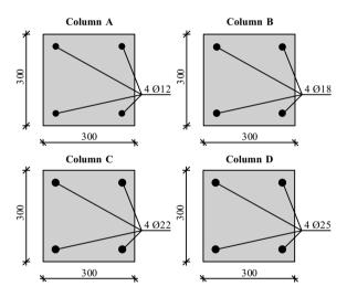
Fig. 6. Cross-sections of the studied columns
