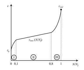
Fig. 4. Variation of concrete deformations with number of cycles
