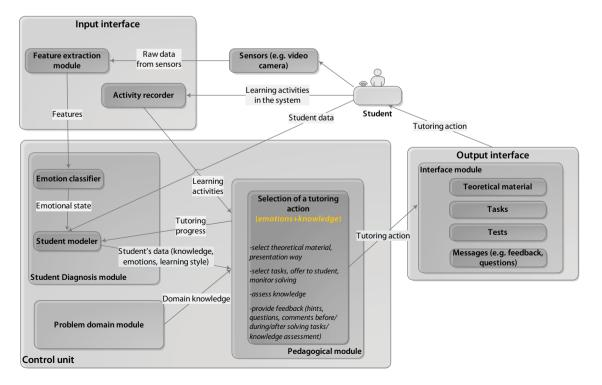
Fig. 2. The overall architecture of the proposed EITS
