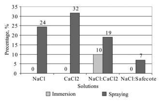
Fig. 4. Percentage rate of stainless steel corrosion product cover by immersion and spraying methods
