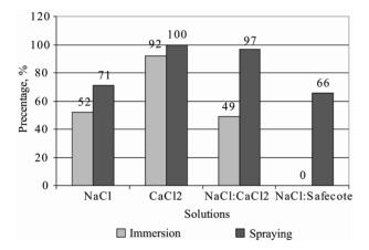
Fig. 3. Percentage rate of carbon steel corrosion product cover by immersion and spraying methods
