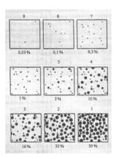
**Fig. 2.** The visual metal specimen's assessment by using a standard picture (Šulčius 2006)
