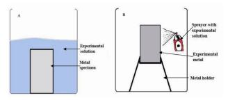
**Fig. 1.** Laboratory experiments. A – Immersion method; B – Spraying method
