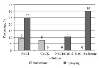
Fig. 5. Percentage rate of galvanized steel corrosion product cover by immersion and spraying methods
