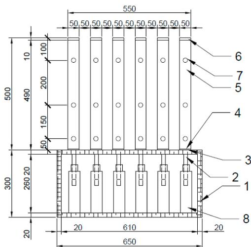
Fig. 1. Stand for a column leaching test: 1 – wooden frame, 2 – tap, 3 – plastic filter, 4 – metal mesh, 5 – organic glass cylinder, 6 – plastic lid, 7 – channel with rubber tube, 8 – 1000-mL HDPE bottle
