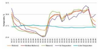
Fig. 15. Shadow effect on the temperatures of the air, water and layers of diesel (shadow from 11:37 till 11:41)
