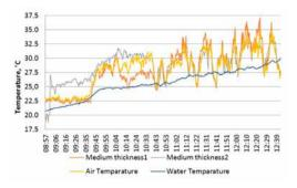
Fig. 5. Temperatures of air, water and the layers with a medium thickness of diesel
