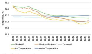
Fig. 18. Differences between temperatures of air, water and diesel layers in the second row
